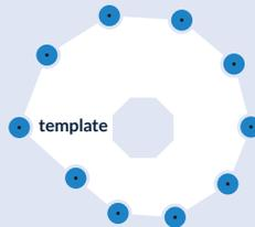
Define the space of the FLOWER by using ground template. Install retractable central pole and perimeter stands. Perimeter stands can be fixed to the ground, or weighted by using water ballast bags (weight from 170kg per stand). There are triangle water ballast bags included in a base platform of central pole too.
